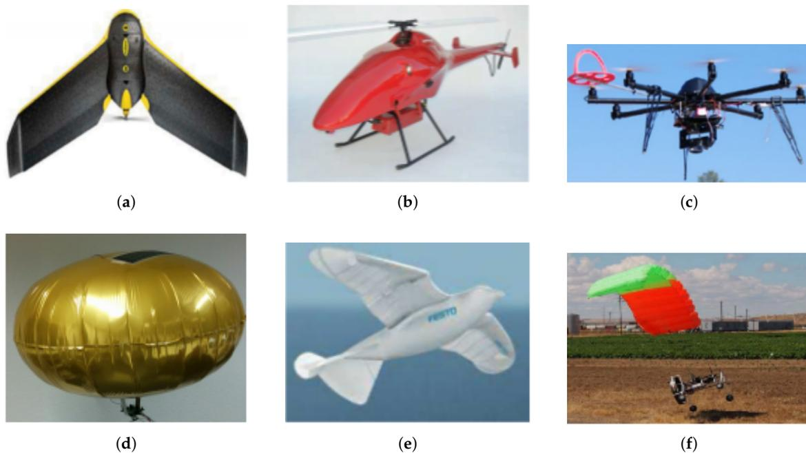
**Figure 1.** (a) Fixed-wing (eBee™) [23]; (b) helicopter (Hornet Maxi) [122]; (c) octocopter [25]; (d) blimp [123]; (e) flapping-wing (SmartBird) [122]; and (f) parafoil-wing (Tetracam) [90].
