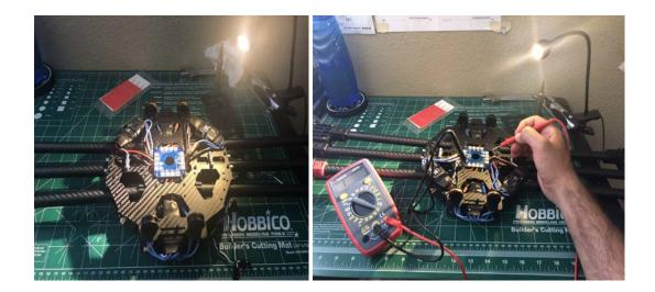
Step 8: mark each motor by number according to the motor rotation of the Hexocopter
