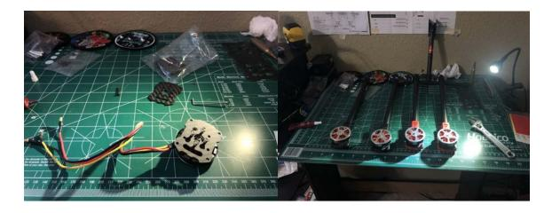
Step 4: connect the remaining four arms to the frame with the carbon fiber pipe buckle
