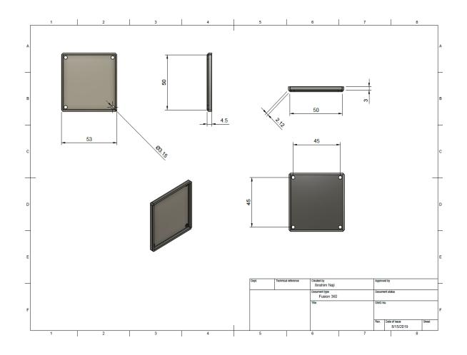
Schematic diagram showing the circuit board cover
